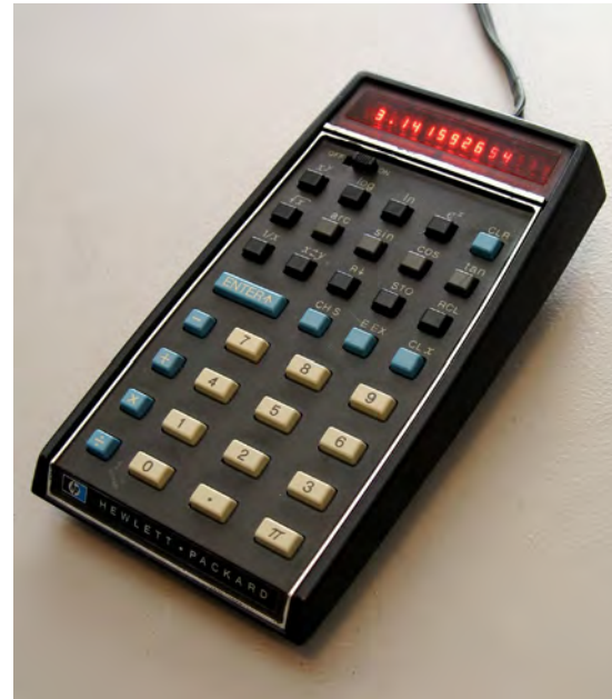
HP-35, the world's first scientific pocket calculator, was introduced in 1972 by Hewlett-Packard. $395,00
